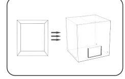
Open the package, there are 12 tubes, 8 connectors,insert 3 tubes of different lengths into a connector, and then connect them one by one.
