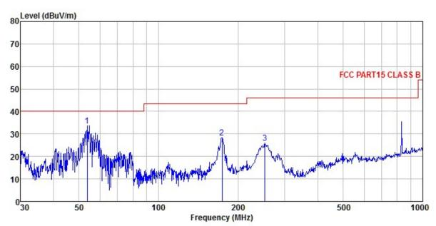
Site Condition : 3m chamber : FCC PART15 CLASS B 3m VERTICAL
