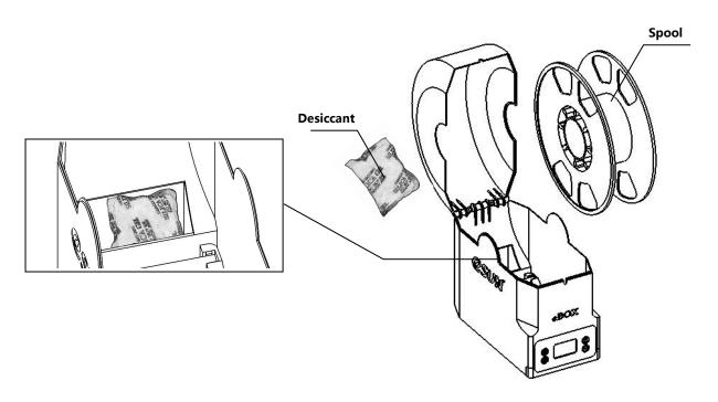
**4.**Put the spool in and pull the filament out through the outlet, close the cover. (The direction to pull filament can be bottom-up, or from top to bottom, depending on the position of printer)
